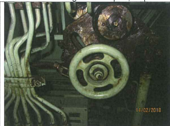
Select clutch for Remote or Local control on Local control stand.
