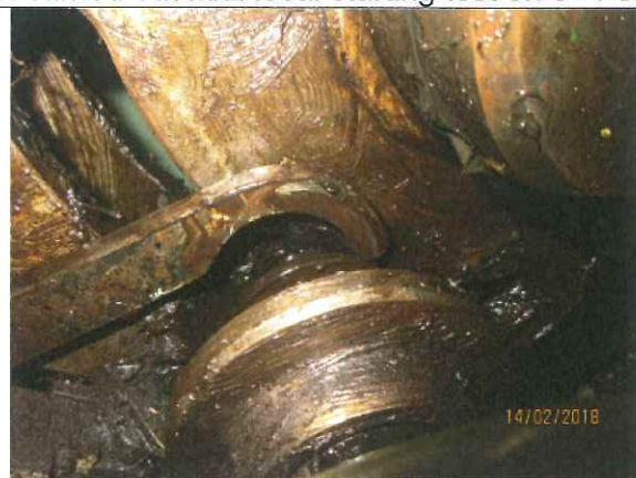
Released locking device and loose clutch (not tighten properly)
