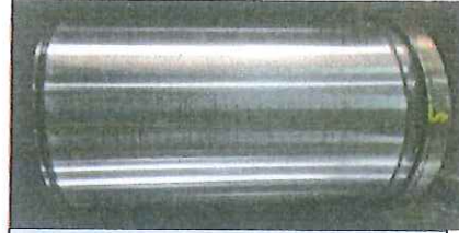
After Polish the Shock Absorber Piston
