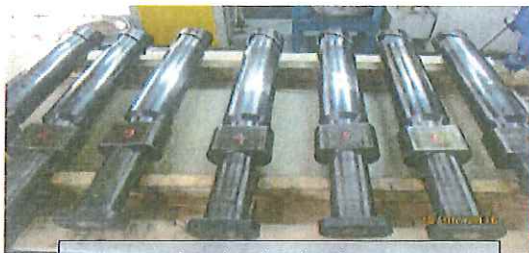
After cleaning the Plunger
