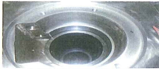
After cleaning the Pump Body
