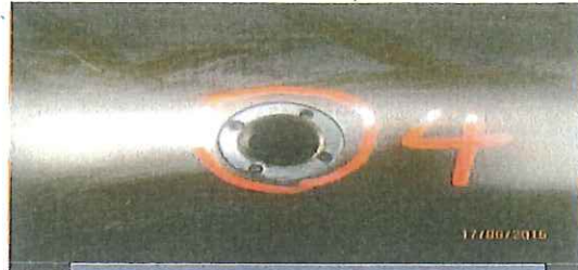
Found #4 Barrel Orifit missing
