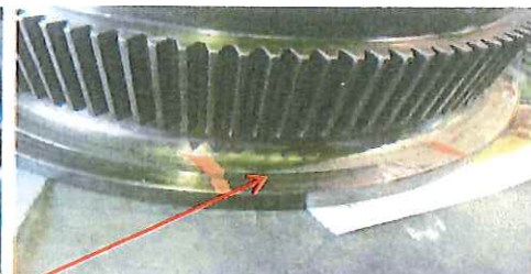
Found all Timing Guide contact surface worn down
